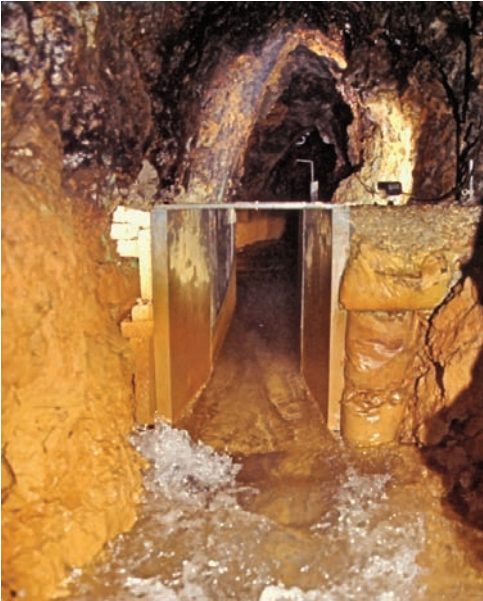
Fig. 58. Parshall flume in the flooded South Crofty/Cornwall/UK tin mine.
