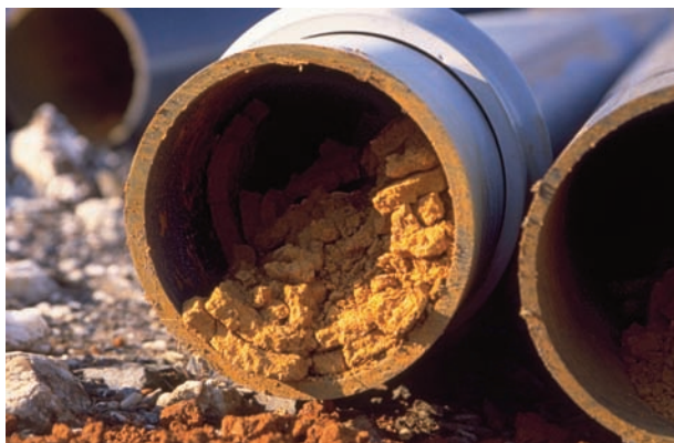
Fig. 8. Ochre precipitates in a mine water discharge pipe of the abandoned Straßberg/Harz fluorspar mine.
