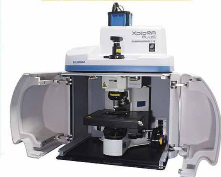
Figure 3: (Left) Raman spectra recorded on different polymer families. (Top right) Aluminum strip pellet containing 12 tablets sent to participants, that were to be dissolved in analytical grade water to control background contamination. (Bottom right) HORIBA Xplora PLUS Raman microscope with class I laser enclosure used for this study.
