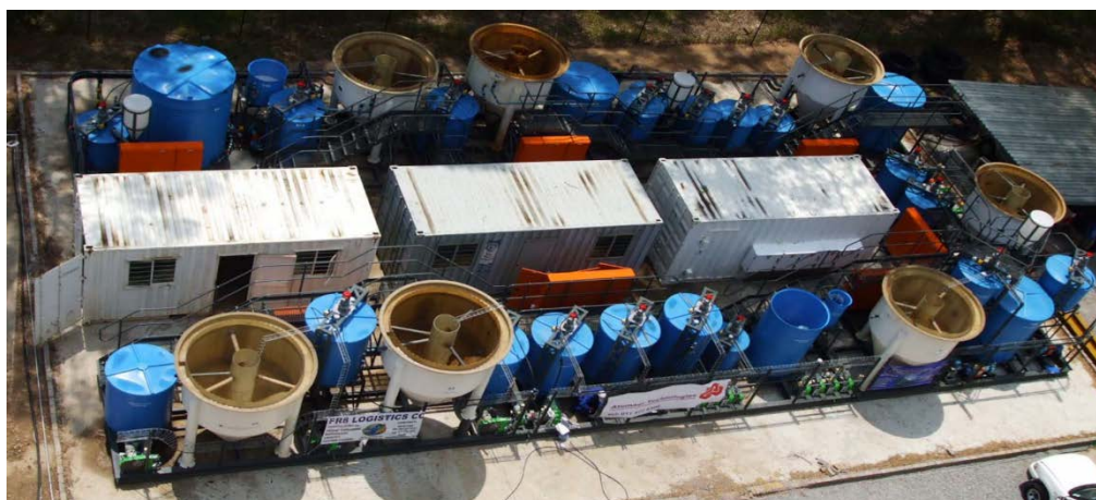
Abbildung 57: SAVMIN™-Pilotanlage am Mogale-Goldbergwerk der Western Utilities Corporation in Südafrika. (Aus Roger Paul: „Presentation to the Parliamentary Committee on Water and Environmental Affairs” – 7./8. September 2011).
