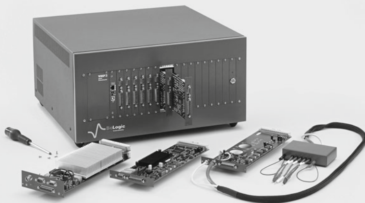
Modular multichannel potentiostat VMP3 manufactured by Bio-Logic (© Biologic SAS)
