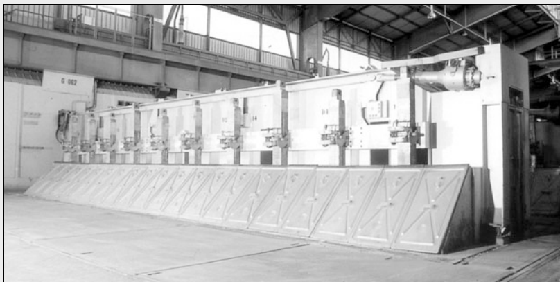
Series of 'AP 30' cells (300 000 A) (© Rio Tinto Alcan, with permission)
